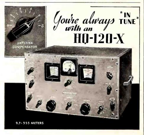
There's a good reason for the high signal-to-notice ratio in the "HQ-120-X." The first tuned circuit of any receiver controls the signal-to-noise ratio. When an antenna is coupled to this very important circuit, there is usually a detuning effect. This detuning effect lowers the signal-to-noise ratio. The antenna compensator on the "HQ-120-X" provides a control for restoring resonance, regardless of the effects of the autenna system. In high galu, highly selective circuits, this coutrol becomes
