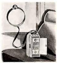
★ A feature of Sentinel's new 3-way "Lightweight Champion"— 247-P is an "Ex-tenna loop" for use in planes, trains, autos and locations where an external antenna is needed. Has 5 tubes, superheterodyne circuit and built-in loop. P.M. dynamic speaker. Tunes 539 to 1550 kc. Plastic tenite case, leatherette trim. Sentinel Radio Corp., 2020 Ridge Ave., Evanston, Ill.—Radio TODAY.
